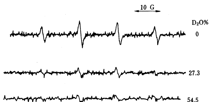
Fig. 3. Effect of D 2 O on DMPO-OH Adduct Formation Mediated by the Decomposition of 4-Ethoxy-1,4-dihydro-2,3-benzodioxin-1-ol ( 1b )
